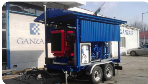
Well Starter Compressor
